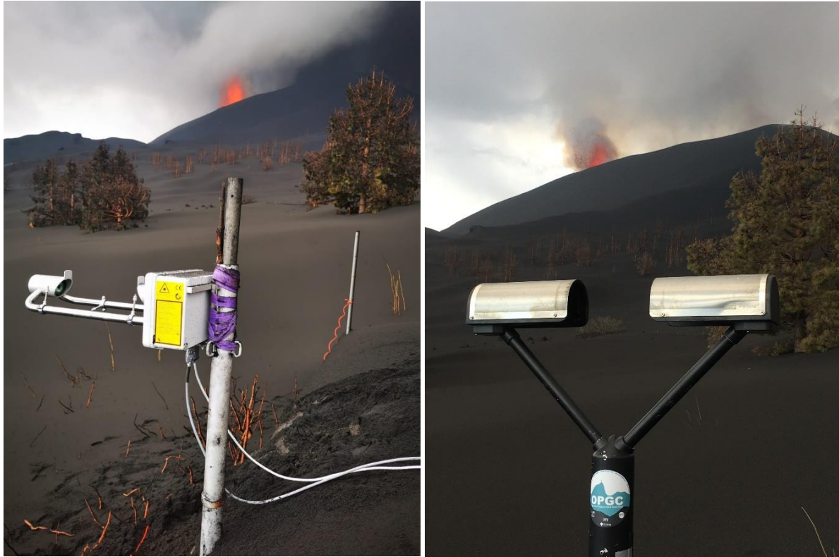
Fig.3 LPM (left) and Parsivel2 (right) disdrometers of OPGC.
