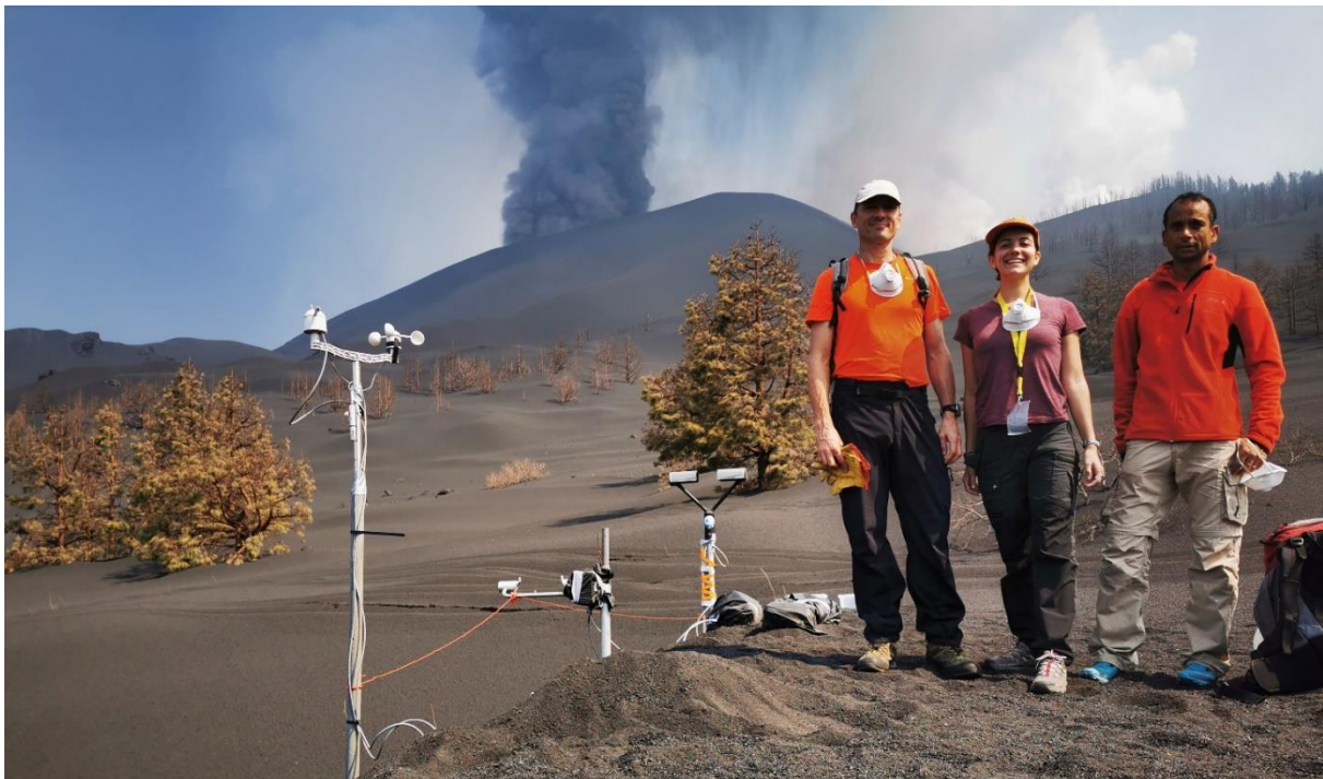
Photo : OPGC-UCA team (F. Donnadieu, C. Biensan, T. Latchimy) next to the instruments deployed 1 km SW of the Cumbre Vieja eruption site : Parsivel2 (background) and LPM (middle) disdrometers, along with anemometer and humidity probe (foreground).
